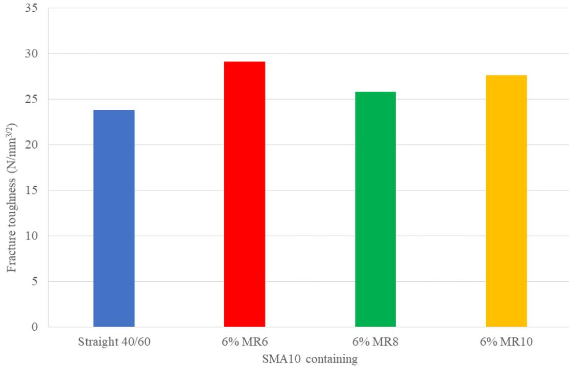
**Figure 6. Asphalt fracture toughness for recycled plastic modified binders**
