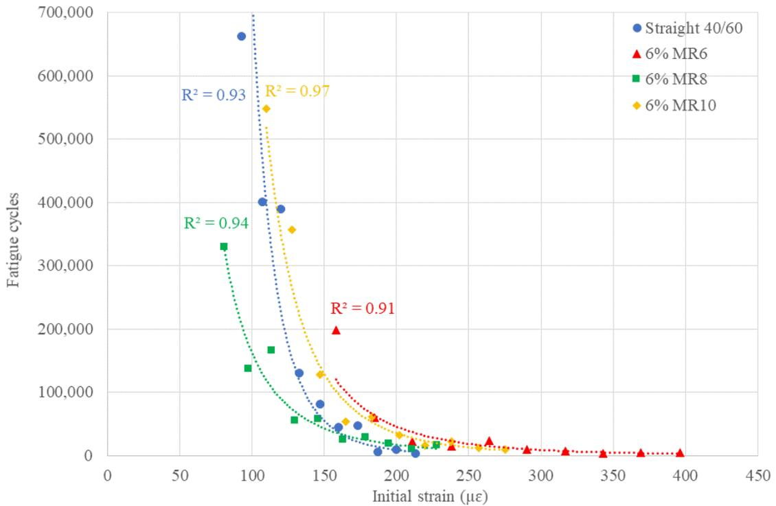
**Figure 7. Asphalt fatigue life for recycled plastic modified binders at different strain**
