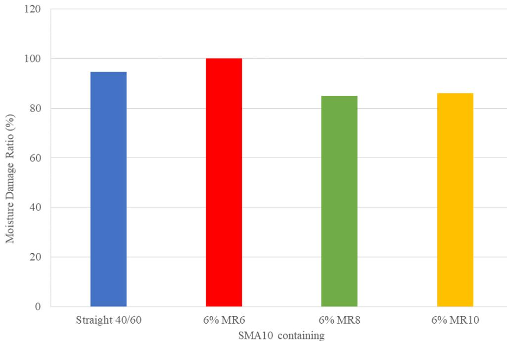
**Figure 2. Asphalt moisture damage ratio for recycled plastic modified binders**
