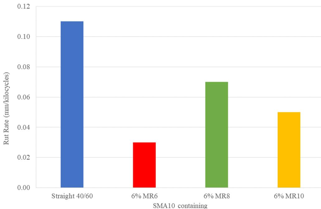
**Figure 5. Asphalt rut rate for recycled plastic modified binders**
