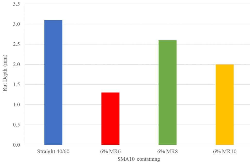
**Figure 4. Asphalt rut depth for recycled plastic modified binders**
