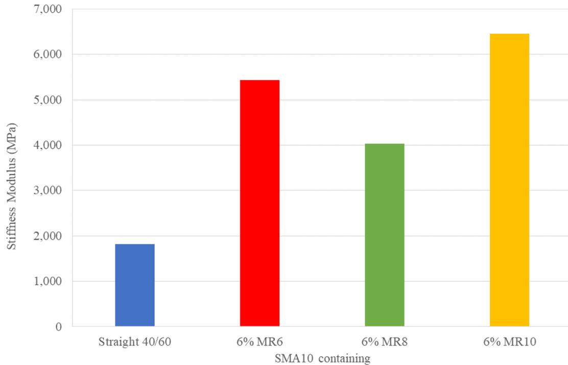
**Figure 3. Asphalt stiffness modulus for recycled plastic modified binders**
